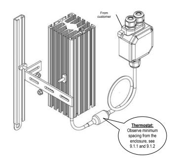
9.1.1 with wiring box provided by the customer inside
