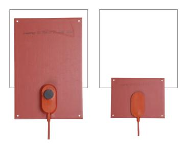
The SSM heater plate can be used for frost protection and as an anti-condensation heater. Its application ensures complete operational safety as the plates prevent malfunctions often due to leakage currents on electrical installations or the corrosion of metal components. Typical applications are switchgear and controlgear cabinets, instrument housings, analyser cases, glove boxes and other enclosures.
